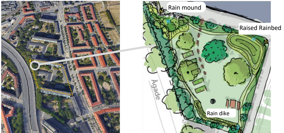
Figure 1: Overview. Left: Demonstration courtyard with roofs to be connected to aboveground NBSsw (dotted line); Right: Stormwater scheme for Zone A with Rain Dike, Rain Mound, Raised Rainbed and 100-y Perimeter Dike (light green line).
